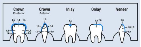
minimum wall thickness in mm
