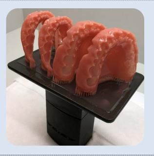
Remove the printed object carefully from the platform
